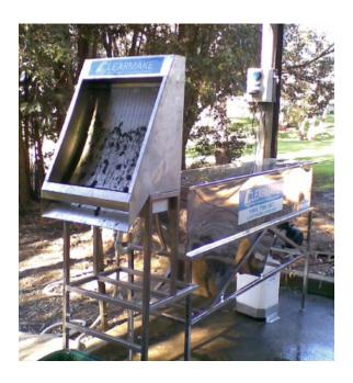
Superior Vertical Tube Coalescing (VTC) technology facilitates improved separation, via the unique spiral tubes, designed to assist in exercising the free floating oils to the surface. These specifically designed VTC blocks also provide optimum flow, serviceability and durability.
